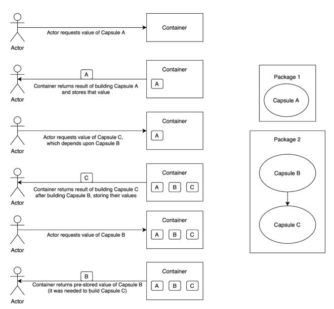
Figure 6: Timeline of container initializing three capsules: A, B, and C, where C has a dependency on B.
