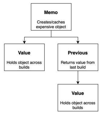
Figure 9: The memo side effect, which creates/caches some object between capsule builds, is composed from two other side effects: value and previous. Value holds the cached object itself, whereas previous is used to track dependencies.
