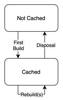
Figure 4: A capsule's life cycle of two states: either cached or not cached. Capsules can be built for a first time, experience rebuild(s), and eventually get disposed.
